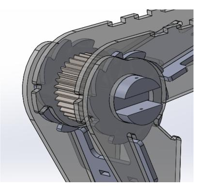
Figure 20 Ratchet Mechanism Design
