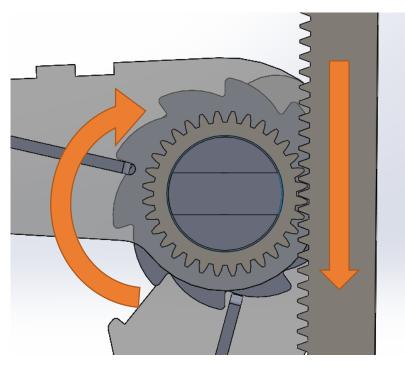
Figure 21: Ratchet and rail combine to depress plunger
