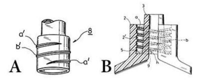
Figure 2: Leur Lok interlocking parts (U.S. Patent No. US6074373, 2000)
