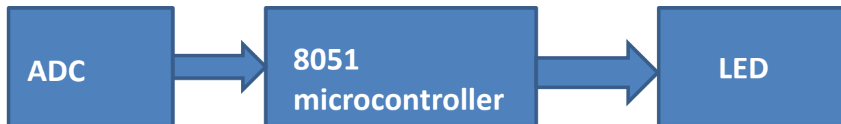
Fig 4: block diagram for interfacing ADC with 8051 microcontroller
