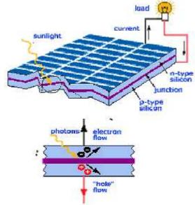
Fig.3.1. Basic structure of PV Cell
