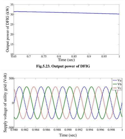
Fig.5.24. Three phase supply voltage of utility grid
