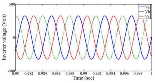
Fig.5.25. Three phase PWM inverter voltage
