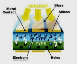
Fig.3.3. Working of PV cell
