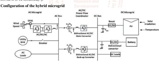
Fig.4.1. A hybrid AC/DC microgrid system
