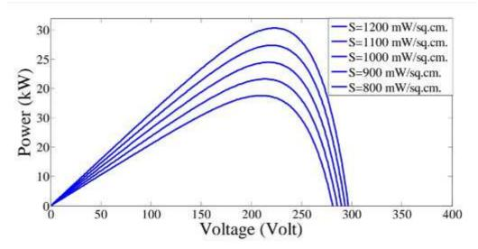
Fig.5.5. P-V characteristics of PV array for different irradiance levels
