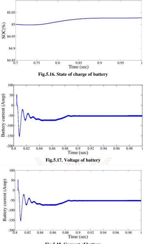
Fig.5.18. Current of battery
