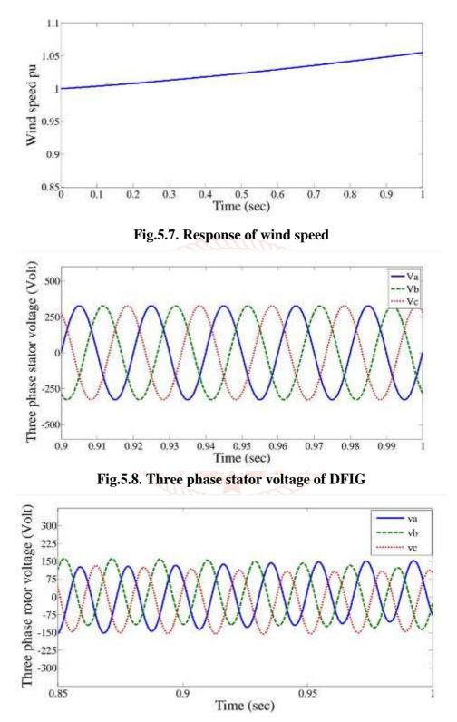
Fig.5.9. Three phase rotor voltage of DFIG
