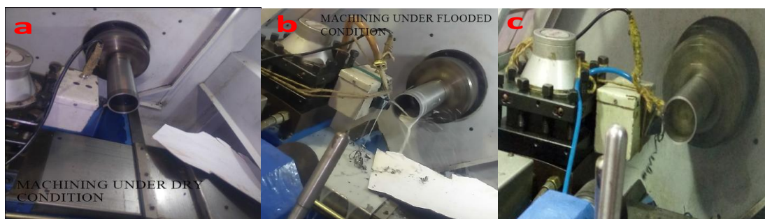
Fig. 3. Cutting environments: a) Dry machining; b) Machining under flooded condition; c) Mist condition
