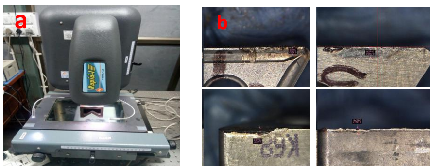
Fig. 4. a) Measurement of tool wear using Z microscope b) Typical results of tool wear using Z Microscope
