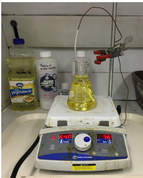
Figure 5: Heating of vegetable oil prior to the addition of alcohol
