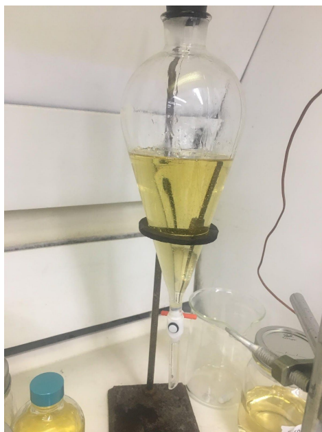
Figure 7: Second stage transesterification separation of methyl esters and glycerol
