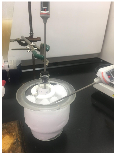
Figure 9: Cooling bath used to conduct cloud and pour point tests on fuel samples
