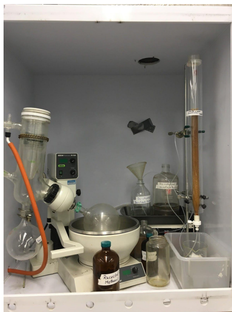
Figure 10: Biodiesel refinery apparatus used to recover excess alcohol and purify esters
