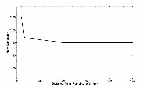
Figure 6. Flow dimension changing with distance from the pumping well, transitioning from radial to subradial.
