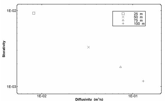
Figure 9. Estimates of diffusivity and storativity showing errors resulting from overestimating cross-sectional flow-path area and underestimating the flow-path length.
