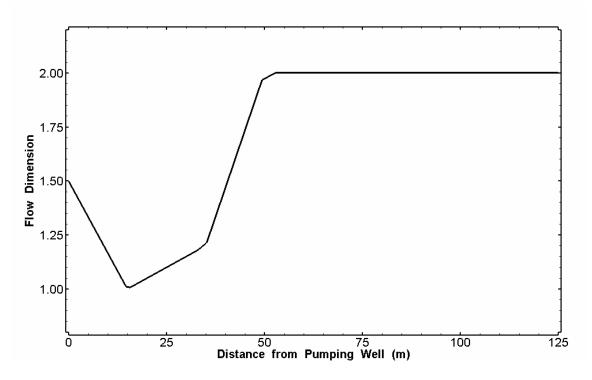
Figure 1. Flow dimension changing with distance from the pumping well, transitioning from subradial to radial.
