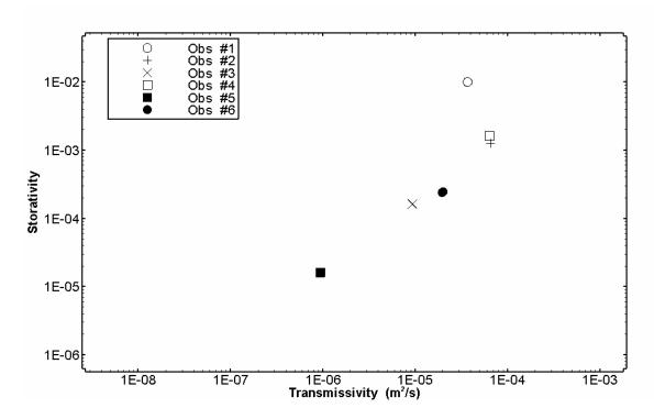
Figure 11. Estimates of transmissivity and storativity obtained from analysis of simulated pumping tests in a two-dimensional binary field.
