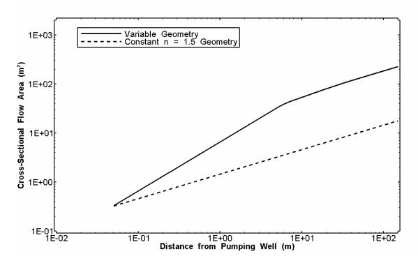
Figure 7. Comparison of cross-sectional flow areas for a variable-geometry model and a model with constant subradial geometry.
