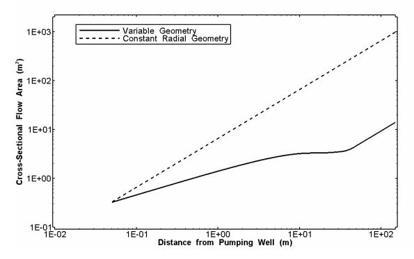
Figure 2. Comparison of cross-sectional flow areas for a variable-geometry model and a model with constant radial geometry.
