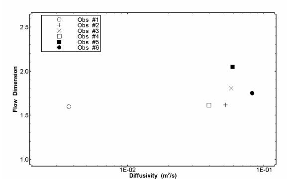
Figure 12. Estimates of diffusivity and flow dimension obtained from analysis of simulated pumping tests in a two-dimensional binary field.
