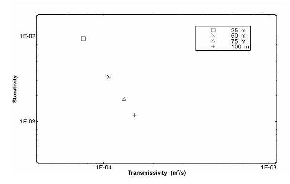
Figure 8. Estimates of transmissivity and storativity showing errors resulting from underestimating cross-sectional flow-path area and underestimating the flow-path length.
