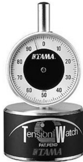
Figure 3.7: Tama Tension Watch used for tuning the drumheads to create reconstructible tensions. Source: www.tama.com
