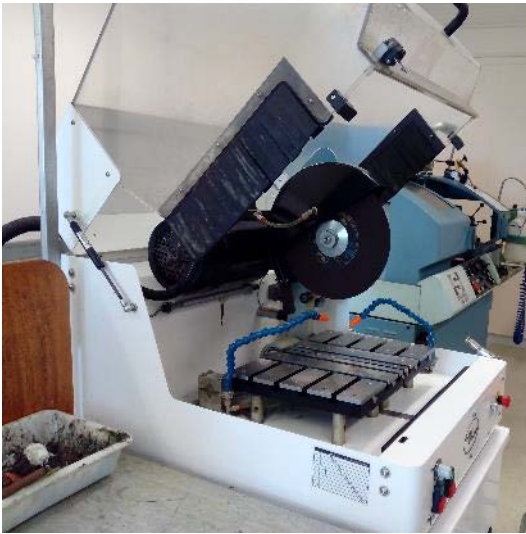
Figure 5: Bench-mounted manual cutting machine. Side view (left) and front view (right).
