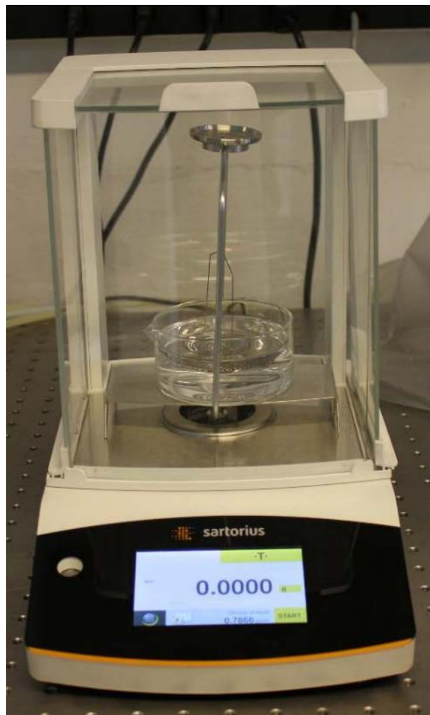
Figure 24: Analytical balance used for the density measurements.
