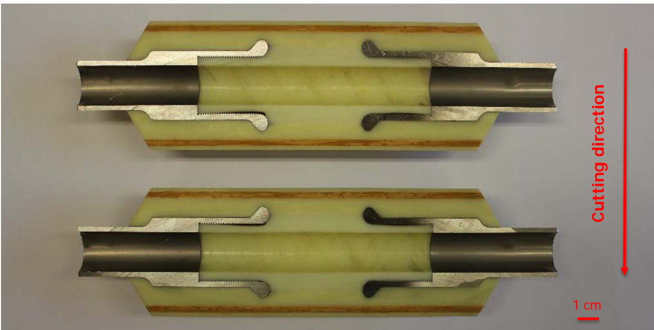
Figure 6: Insulation break after axial sectioning. Cutting direction is shown for reference.
