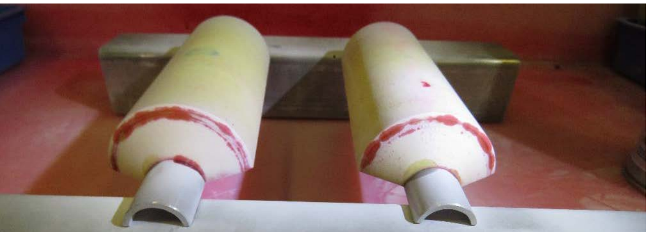
Figure 15: Outer surface of the insulation break after application of developer. Dwell time: 5 minutes.
