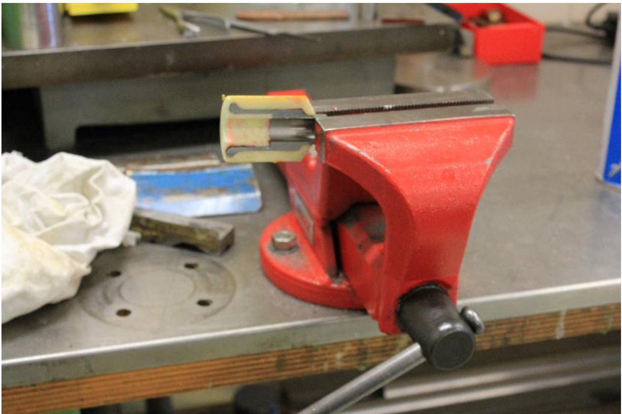
Figure 21: Separation of the inner composite - stainless steel fitting from the outer composite in portion C.
