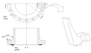
Fig. 1 Typical bolted-flanged joint and wedge model.
