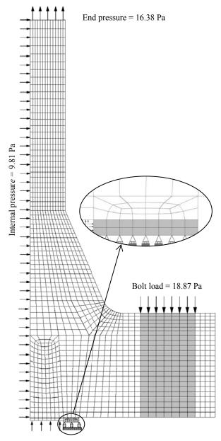
Fig. 5 Axisymmetric finite element mesh.
