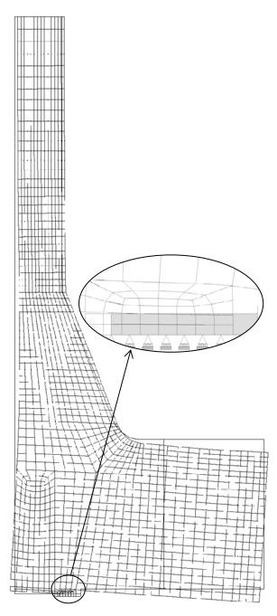
Fig. 7 Deformed flange, step 2, 9 increments, Mag. 100%.
