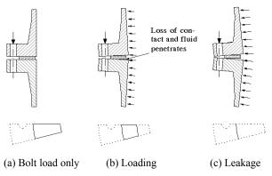
Fig. 2 Contact area at three load increments.
