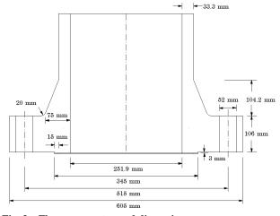
Fig. 3 Flange geometry and dimensions.
