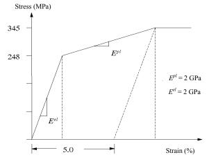
Fig. 4 Gasket stress-strain diagram.
