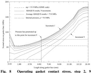
rig. 8 Operating gasket contact stress, step 2, 9 increments.
