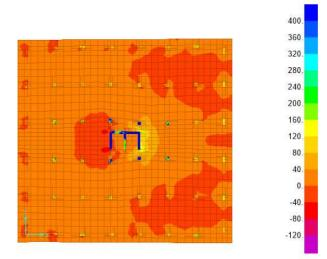
Fig. 3.5.3 BM variations in raft slab for K = 95000 kN/m3 in EQX loading case **Fixed Support**
