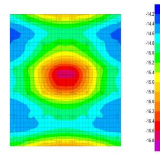
3.2Settlement of raft with spring support K=45000, for load case of 1.0(DL+LL)
