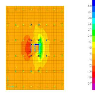
Fig. 3.5.1 BM variations in raft slab for K = 10000 kN/m3 in EQX loading case  $K = 45000 \text{ kN/m}^3$
