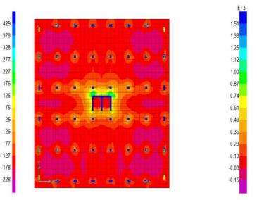
Fig. 3.5.4 BM variations in raft slab for K = 10000 kN/m3 in 1.2(DL+LL+EQX)
