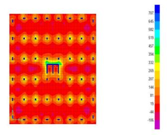
Fig. 3.5.7 BM variations in raft slab for fixed supports in 1.2(DL+LL+EQX)
