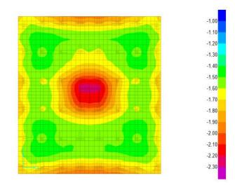
3.4 Settlement of raft slab with fixed support for load case of 1.0 (DL+LL)
