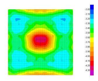
3.3 Settlement of raft with spring support K=95000, for load case of 1.0(DL+LL)
