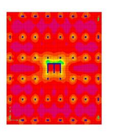
Fig. 3.5.6 BM variations in raft slab for K = 95000 kN/m3 in 1.2(DL+LL+EQX)
