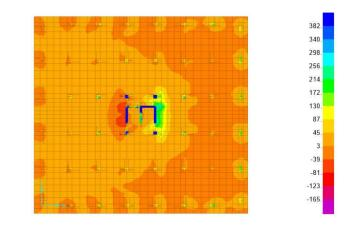
Fig. 3.5.3 BM variations in raft slab for fixed supports in EQX loading case
