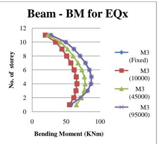
2.4Bending Moments at Support of Beam connected with Exterior Column
