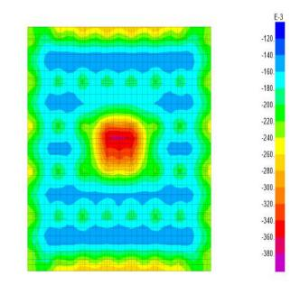
3.5 Bending Moments in the Raft Slab along X-Direction (MX)
