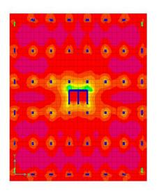
Fig. 3.5.5 BM variations in raft slab for K = 45000 kN/m3 in 1.2(DL+LL+EQX) K = 95000 kN/m<sup>3</sup>
