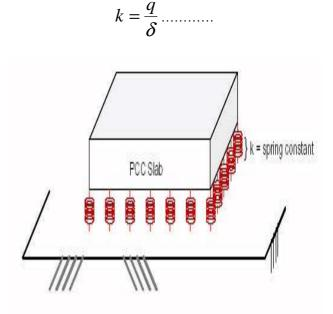
Fig. 1.1 Modulus of Subgrade Reaction
