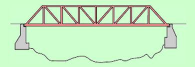
• **Howe** - The Howe truss is the opposite of the Pratt truss. The diagonal members face in the opposite direction and handle compressive forces (requiring thicker elements. This makes it very uneconomic design for steel bridges and its use is rarely seen.
