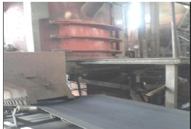
Fig.5: Dry Sand on Belt Due to Excess & Mixer Door Clearance between Mixer Door & Mixer
