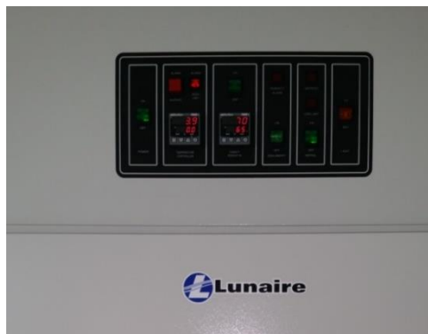
Fig. 5. Main control panel (testing conditions: H=65%, T=0° C)
