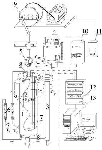
Fig. 1. Experimental set-up: 1 - tubular vessel, 2 - perforated plate agitator, 3 - external overflow, 4 - generator of input temperature signal and hot liquid feeder,
