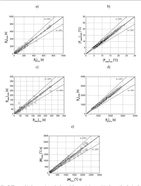
Fig. 5. The graphical comparison of values of characteristic quantities for results obtained experimentally and using ANN model: a) the time lag of thermal process -  $t_0$ , b) the maximal value of temperature -  $T_{\max}$ , c) the time of the achievement of maximal value of temperature -  $t_{\max}$  d) the time duration of thermal process -  $t_p$  and the e) quantity of area between the thermal response of transient process and the time axis - A
