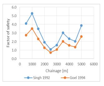
Figure 2 Results showing Factor of safety from Singh's approach and Goel's approach.
