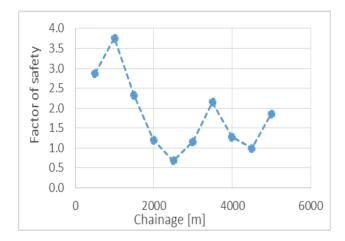
*Figure 3:* Graph showing chainage against Factor of safety from Jethwa et al. approach
