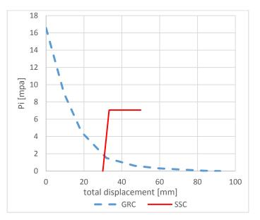
**Figure 5:** Ground reaction curve (GRC) and Support characteristic curve (SCC) plotted in same graph to determine stability of tunnel section against squeezing.
