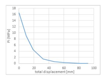
Figure 4 Ground responsive curve for tunnel section at 2+500m
