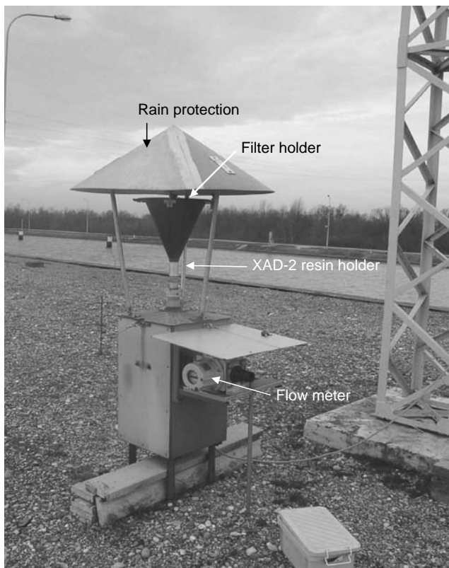
FIGURE 10.1 High-volume sampler developed in the LPCA. (From Scheyer, A., PhD thesis, University of Strasbourg, 2004.)
