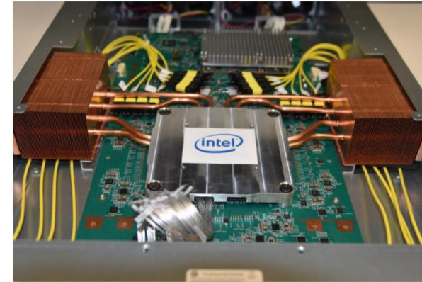
Intel's Demo Co-Packaged Optics Ethernet Switch Vehicle
