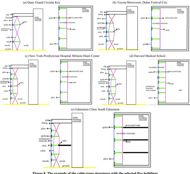
Figure 8. The example of the cable-truss structures with the selected five buildings
