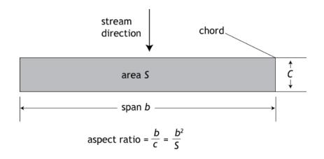
Demonstrate that the current definition of the aspect ratio of a wing coincides with the earlier definition when the wing was rectangular.
