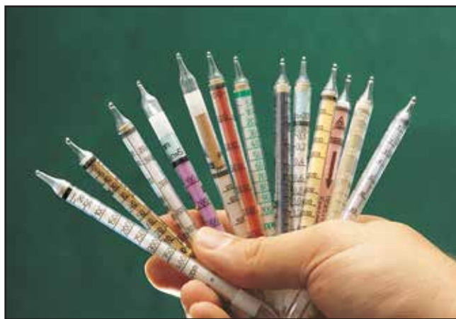
Figure 6.10 Colorimetric tubes will show different colors based on the detection of specific chemicals. Courtesy of MSA.
