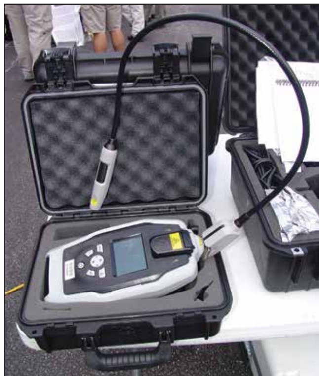
Figure 6.31 Raman spectroscopy uses a high intensity light, such as a laser, to identify materials.
