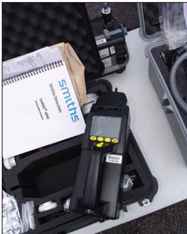
Figure 6.27 Ion mobility spectrometry can help identify some materials that are difficult to detect via other methods.
