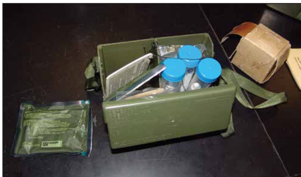
Figure 6.17 The M256A1 Detector Kit can be used to detect airborne WMD agents.
