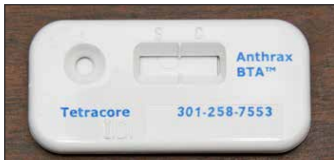
Figure 6.21 Immunoassay indicators are used to detect a reaction to a biological agent.
