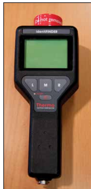
Figure 6.29 A gamma-ray spectrometer identifies the activity level of a source.
