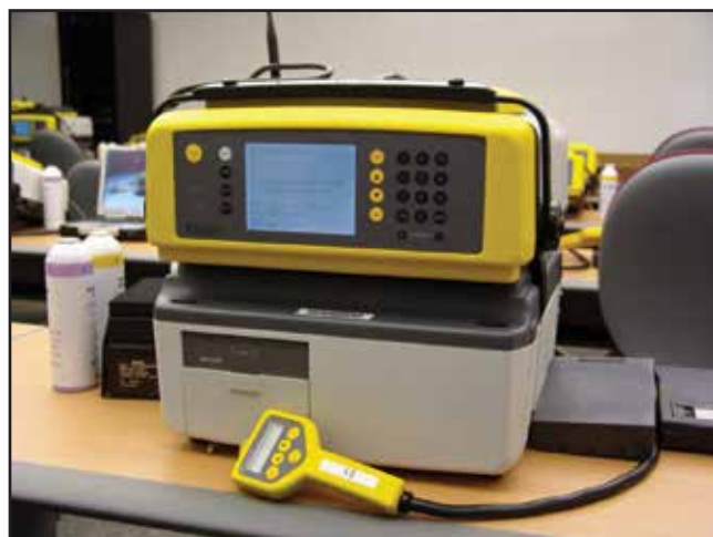
Figure 6.26 GC/MS equipment has become more portable over time, but the results must still be analyzed and interpreted.
