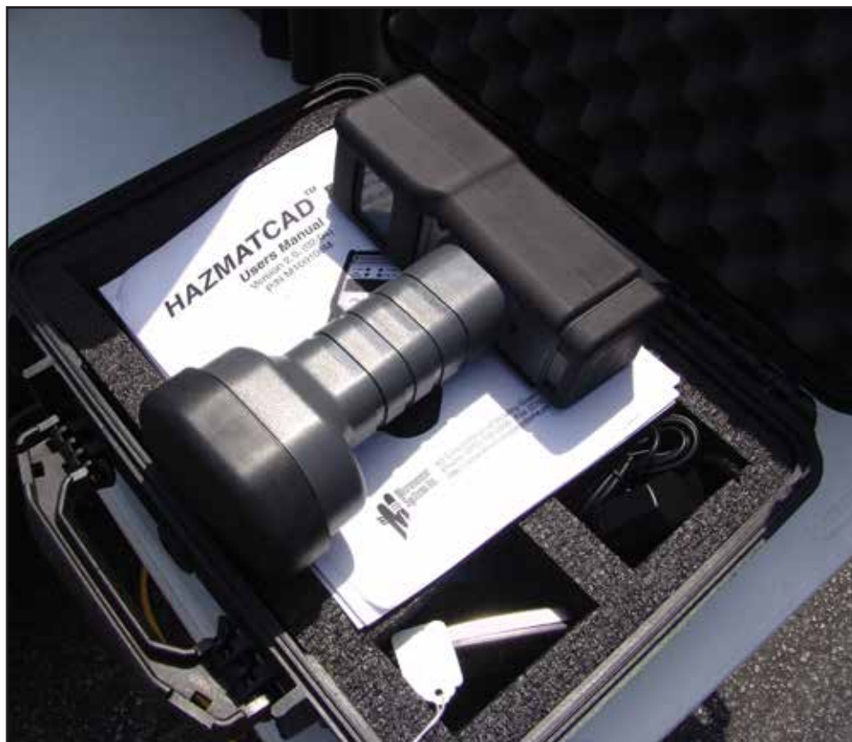
Figure 6.28 Surface acoustic wave sensors may be helpful in detecting nerve and blister agents.
