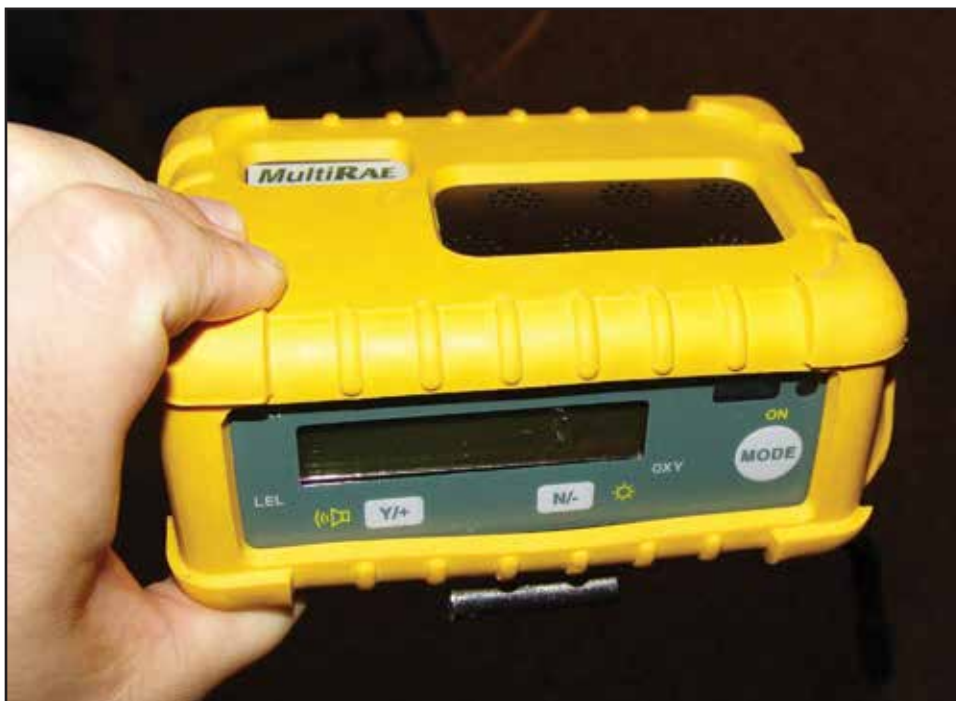
Figure 6.7 Combustible gas indicators may work reliably in oxygen-deficient atmospheres.
