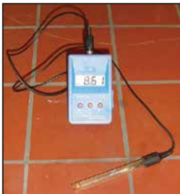
Figure 6.9 pH meters must be calibrated for accuracy.
