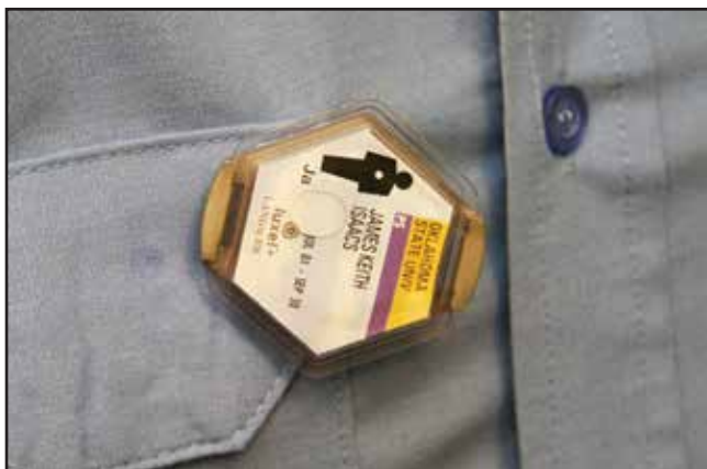
Figure 6.4 Badge dosimeters typically display the absorbed radiation dose.
