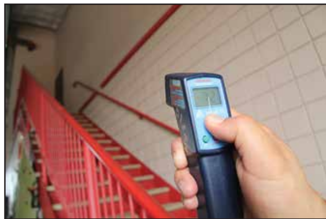
Figure 6.23 Infrared thermometers can sense temperature without contacting the material.
