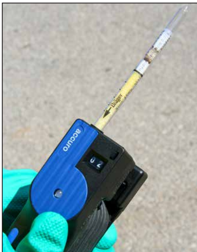
Figure 6.11 The length of the stained section will indicate the concentration of the detected contaminant.
