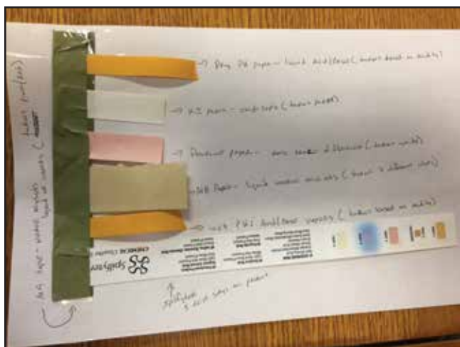
Figure 6.16 This array of test strips includes a wastewater detector strip. Courtesy of Scott Kerwood.
