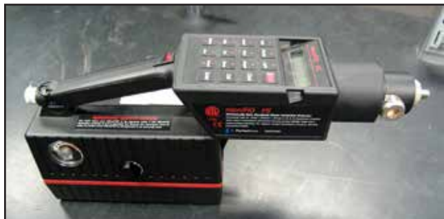
Figure 6.24 Flame ionization detectors can return results on nearly all organic compounds.
