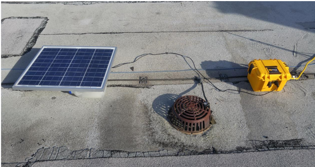
Figure 30. Basic setup for a GP3L Test System (second panel not shown)
