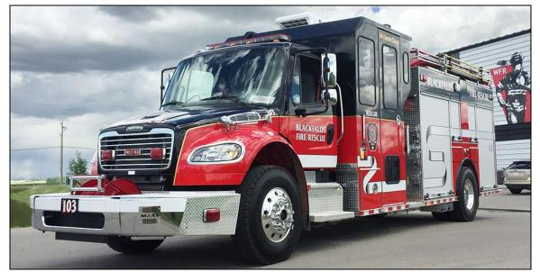
Blackfalds, AB got this 2017 Freightliner M2-106/Pierce product last year. Rescue 103 has a 1500gpm Hale pump, 1200gwt, 30gft, and a FoamPro 2002 foam system. (Wholesale Fire & Rescue)
