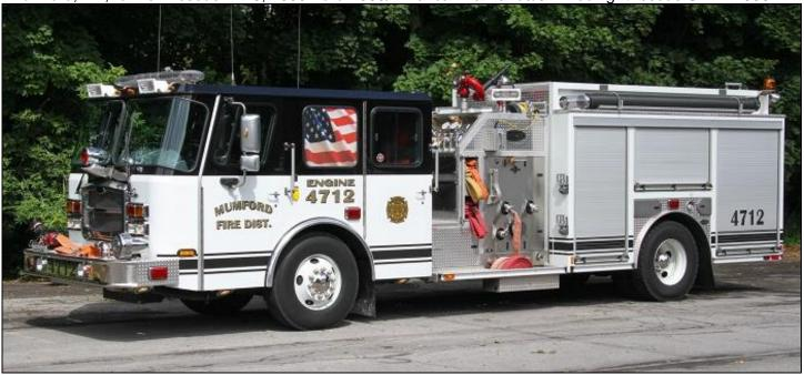
Mumford, NY Engine 4712, a 2011 E-One Typhoon with a 1500gpm pump and a1000gwt. SN 136439. (lan Duke photos)
