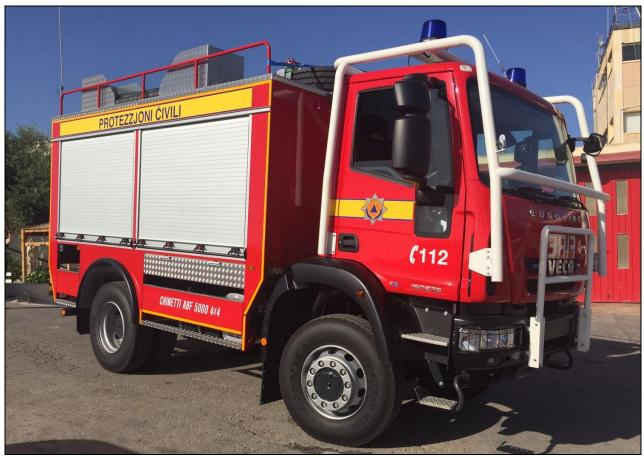
Some new appliances for Malta: a 2017 Chinetti water carrier on an Iveco 4 x 4 chassis. It carries 5000 L water with a 2000 I/min Chinetti pump.
