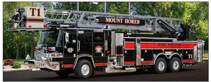
Mt. Horeb, WI is known for their all black apparatus. Truck 1 is a 2016 Pierce Quantum quint with a 1500gpm pump, 500gwt and an 85' rear-mount tower. SN 29367.
