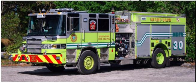
Miami-Dade, FL has a distinctive grey over lime set up. Engine 30 is a 2008 Pierce Arrow XT pumper with a 1500gpm pump and a 750gwt. (Pierce Fire Apparatus photo)
