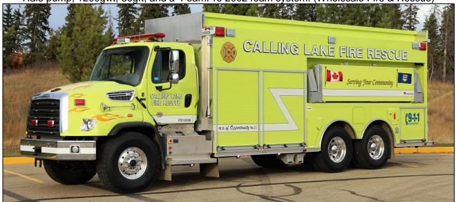
Calling Lake AB, recently put this 2017 Freightliner M2-114SD/Rosenbauer tanker in service with a 1050igpm Rosenbauer pump, and a 3000gwt. s/n 21654. (John Bowerman photo)
