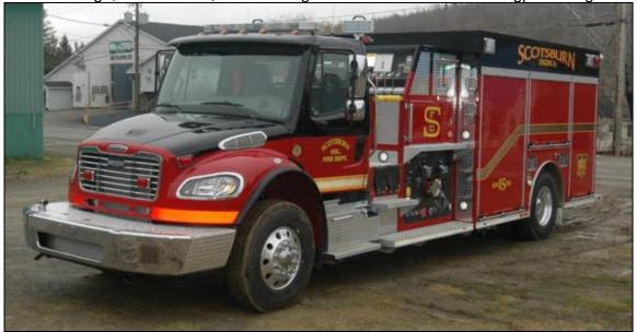
Scotsburn, NS Engine 15, a 2017 Freightliner M2-106 / Metalfab 1250igpm/1000gwt/25gft. FoamPro 2001 FS (Metalfab Fire Photos)
