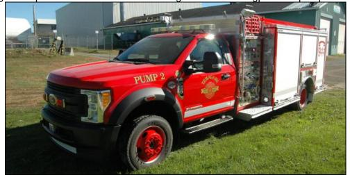
Temagami Pump 2, a 2017 Ford F550 4x4/Metalfab light pumper with 1050igpm Hale pump, 300gwt and FoamPro 1600 foam system. (Metalfab Fire photos)
