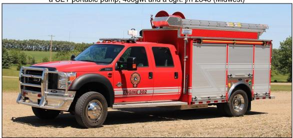
An Acres rig from 2017, this one for Transcona, MB. Uint 302 was built on a Ford F550 4x4 chassis with a 1050igpm Waterous pump, 500gwt and 20gft. s/n #170127149.
