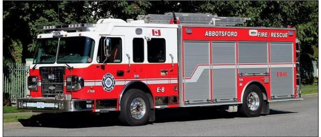
Abbotsford, BC Engine 8, a 2016 Spartan Metro Star/Hub pumper with a 1750igpm Hale pump, 500gwt and 50gft. (Shane MacKichan photo)
