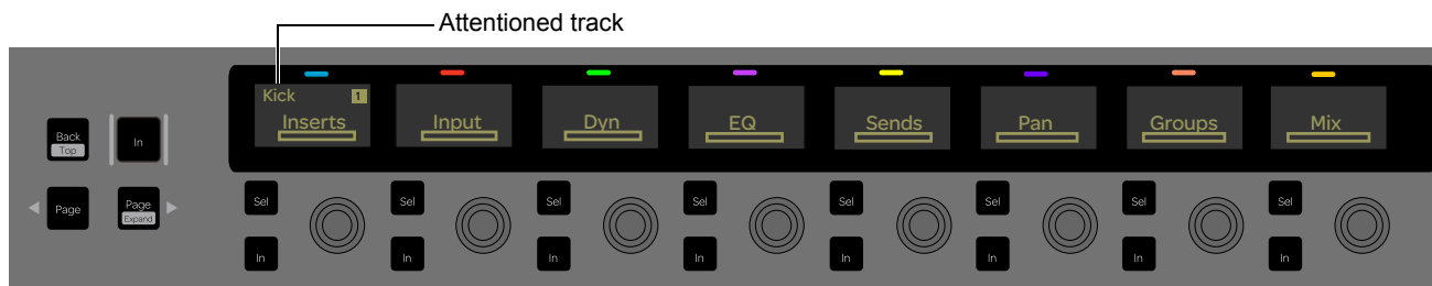
Channel Control top-level Knob Set, showing the attentioned track in the leftmost display
