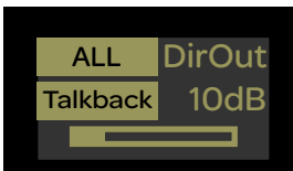
Encoder display for an S3 audio input showing it assigned as the Talkback input source
