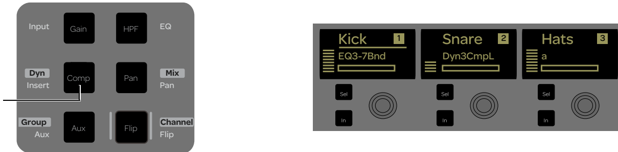
Insert switch (left); Channel displays showing the first Inserts slots for tracks 1–3
