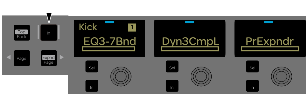
Channel Control Navigation In switch
