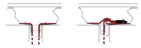
Fig. 24 GM-RAKE downspout hangers
