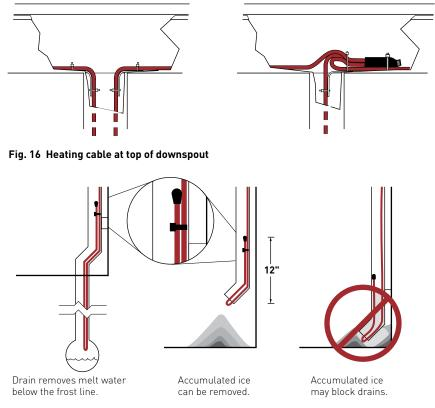
Fig. 17 Heating cable at bottom of downspout
