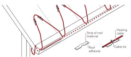
Fig. 21 Belt loop approach on a sloped roof
