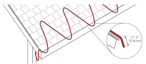
Fig. 10 Layout for heated drip loops
