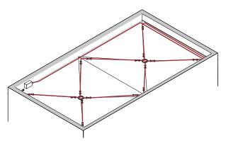
Fig. 22 Belt loop approach on a flat roof
