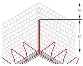
Fig. 12 Layout for a roof valley
