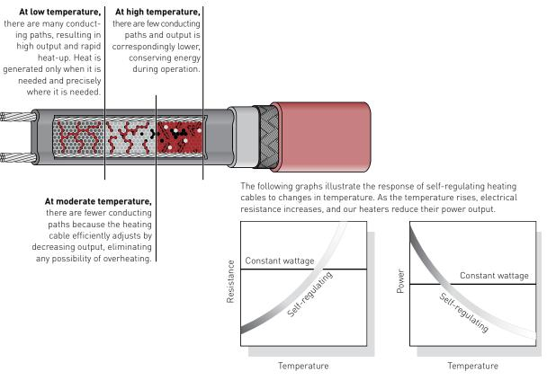
Fig. 3 Self-regulating heating cable technology
