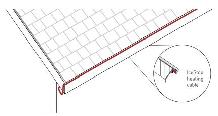
Fig. 11 Layout for heated drip edge
