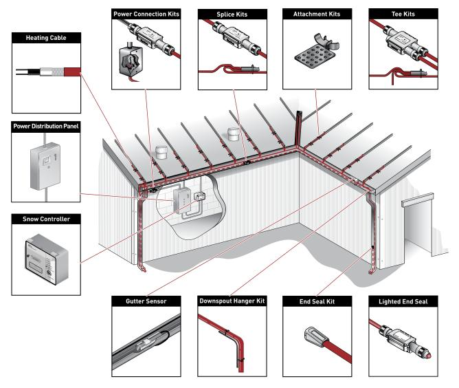
Fig. 1 Typical IceStop roof and gutter de-icing system
