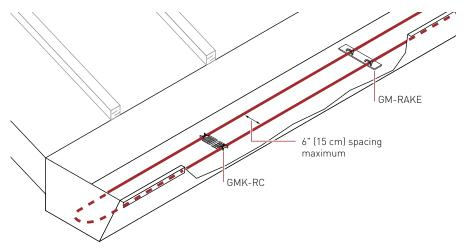
Fig. 23 GMK-RC clip in a gutter
