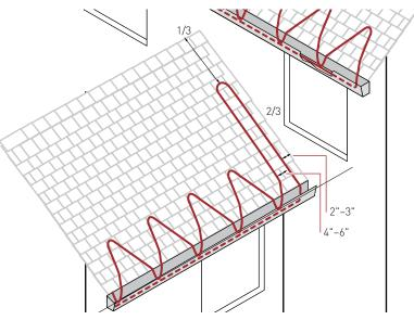
Fig. 13 Layout for a roof/wall intersection.
