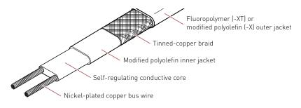
Fig. 2 IceStop heating cable construction
