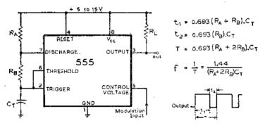
Fig, 7. Astable Operation Of 555 Timer.
