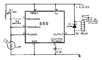
Fig. 29. Light Operated Relay
