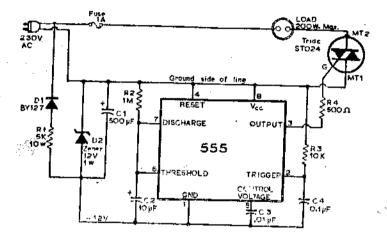
Fig. 24. Circuit Turns Power On After Delay
