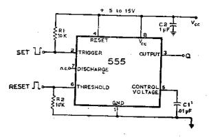
Fig. 10. 555 Timer Operated As A Flip Flop.
