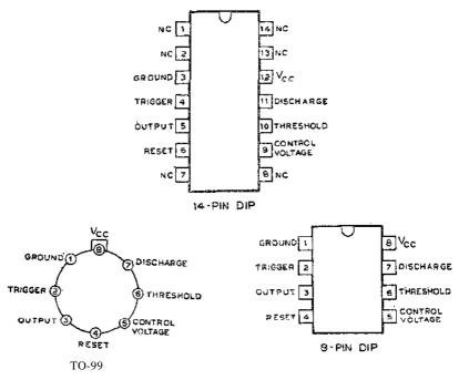
Fig. 1. Pin Connections For The 555 Timer. (TOP-VIEWS)
