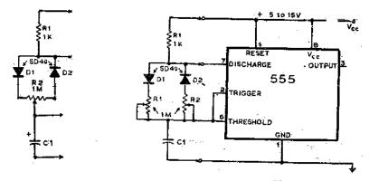
Fig. 9. Independent Control Of Charge And Discharge Timings.
