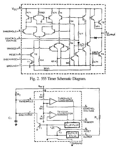
Fig. 3. Functional Block Diagram.
