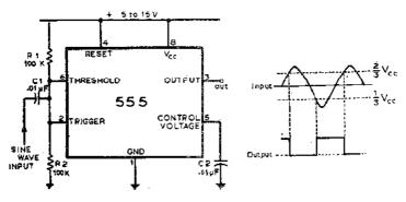
Fig. 11. 555 Timer As A Schmitt Trigger.
