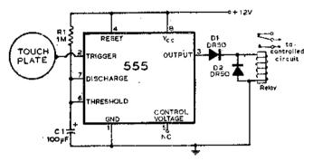
Fig. 14. Touch Controlled Relay.
