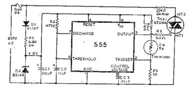
Fig 30. Temperature Controller
