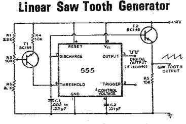
Fig. 20. Sawtooth Generator Using Current Source
