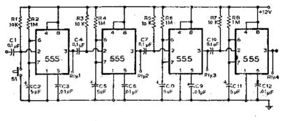
Fig. 32 Sequential Switching,
