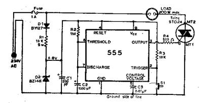
Fig. 23. Circuit Turns Off Power After Delay,
