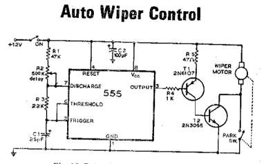
Fig. 15. Delayed Auto-Wiper Cycle Timer
