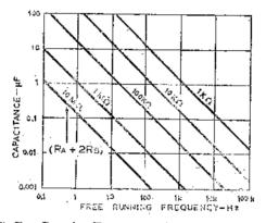
Fig. 8. Free Running Frequency Of Astable Multivibrator.
