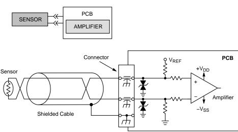
Figure 13. Remote Sensor Circuits are an Example of an Application that Can Benefit from the Symmetrical Clamping Feature of a Bidirectional TVS Diode
