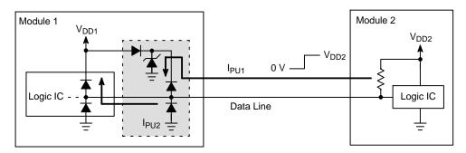
Figure 11. Back Drive Protection can be Implemented by Adding an Avalanche and Blocking Diode to the Diode Array. The Blocking Diode Eliminates the I<sub>PU1</sub> Current Path; However, Current Path I<sub>PU2</sub> will Exist if the IC has a Diode Connected between the Output and Power Supply Pins
