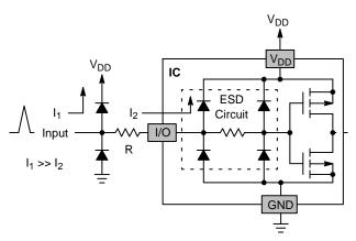
Figure 4. R Forces I<sub>1</sub> >> I<sub>2</sub>, which Ensures that the Majority of the Surge Energy is Diverted by the External Diode Array rather than by the IC's Internal ESD Circuit
