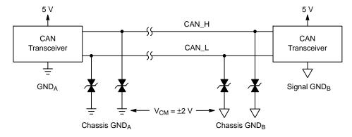
Figure 7. Bidirectional TVS Devices Solve the ±2.0 V Common Mode Offset Voltage (V<sub>CM</sub>) Requirement of CAN Transceivers
