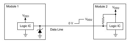
Figure 10. A TVS Avalanche Diode Eliminates the Current Path (I<sub>PU</sub>) for Back Drive; However, the Problem will Still Exist if Module 1's Logic IC Uses a Diode Array for ESD Protection
