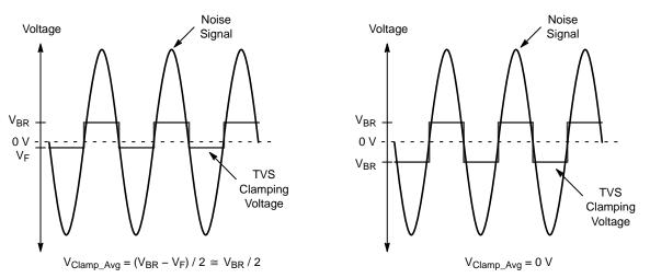
Figure 12. The Average Clamping Voltage of a Unidirectional TVS Diode for a Sine Wave Input is V<sub>BR</sub>/2. The Symmetrical Breakdown Voltages of a Bidirectional Device has an Average Clamping Voltage that is Biased at 0 V
