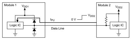
Figure 9. A Diode Array Creates a Back Drive Current Path ( $I_{PU}$ ) to Provide Power through a Data Line when  $V_{DD2} > V_{DD1}$
