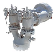
The Anderson Greenwood Tandem Safety Selector Valve System allows for simultaneous selection of pressure relief valve and corresponding discharge outlet piping of dual pressure relief devices discharging into a closed header system.
