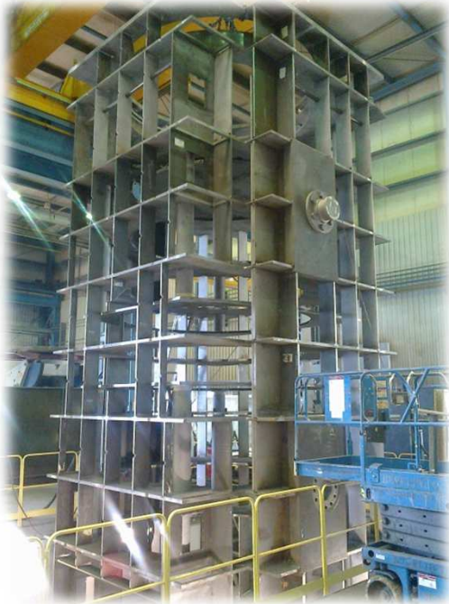
MAC (A63) Generator Casing : weight: 83.200 kg 9.800 x 4.100 x 4.100 mm; material: S355J2+N
