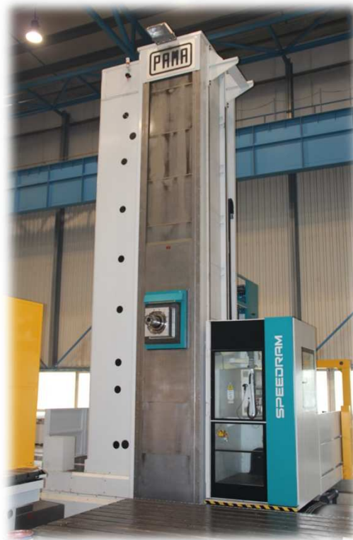
PAMA horizontal boring mill : length 24 m, vertical 6 m, depth 2.6 m
