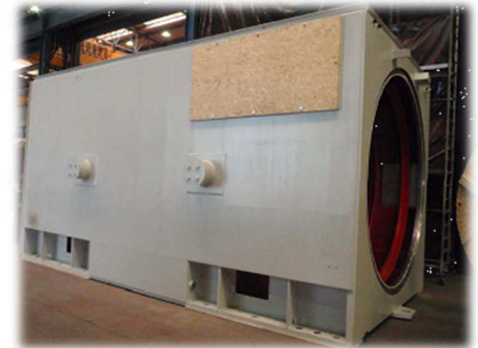
9A5 Generator casing : weight: 44.000 kg 7.050 x 3.585 x 3.585 mm; material: S235J0+N
