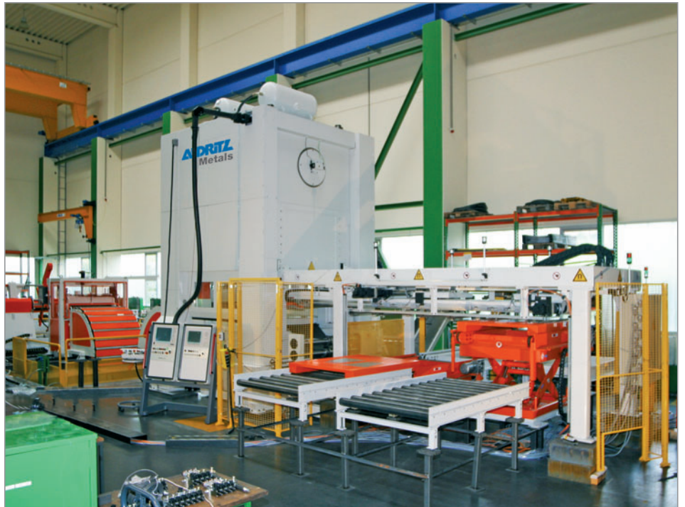
Cutting line for big rotor-stator-laminations.
