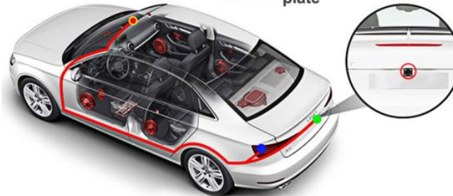
Image 43: Rear camera installation wire diagram
