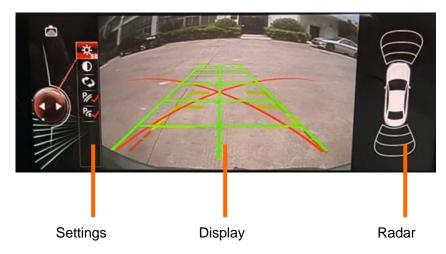
You can settings the Brightness/contrast and the path line/Radar Only can show the display of Radar if the original car with Radar.
