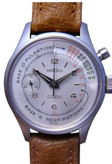
57 - Angelus doctor's dial-chronograph with cal. Valjoux 22, here the mono-pusher version (also made as two-pusher). Some watches have "Medical" on the dial. Here with original crystal with magnifier section.
