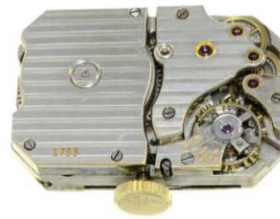
14 - The movement of the Tiffany’s watch in picture 13, the Angelus SF-N 9.
