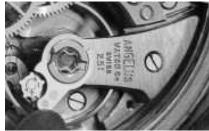
Type 3d (cal. 250-256 with Incastar regulator, the signature without frame: “ANGELUS / WATCH Co / SWISS”, 1948 until ca.1957)
