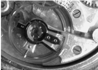
Type 1c (cal. 216, ca. 1940; as type 1b, but with shock protection).
