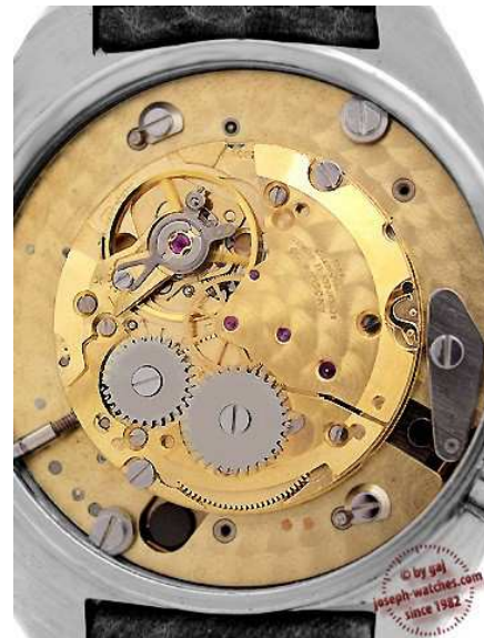
60 - Movement of the repetition wristwatch in picture 59, ETA 2801 with module by Dubois Dépraz, 1976.
