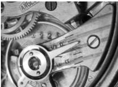
Type 2 (the middle version of cal. 215 and first version of cal. 217, from ca. 1942 until ca. 1950).
