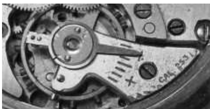
Type 3b (cal. 250-256, 1948 until ca.1957; here with the calibre number, which is not always marked)
