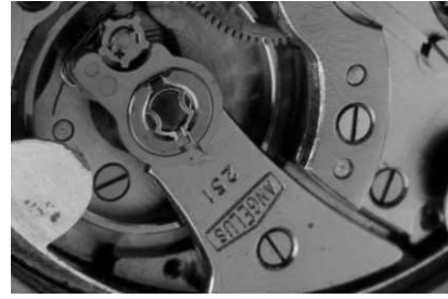
Type 3c (cal. 250-256 with Incastar-regulator, signature „ANGELUS“ in frame, 1948 until ca. 1957).
