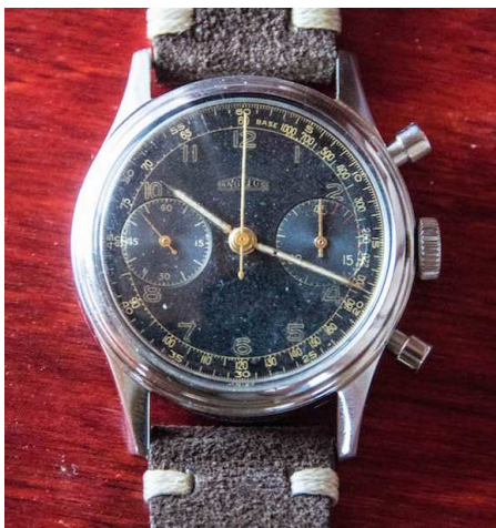
41a - Military chronograph for the Hungarian air force, calibre SF 215, here the version with the seconds scale outside the tachymeter scale (a version with the tachymeter scale at the outside also exists), logo D3, ca. 1951.
