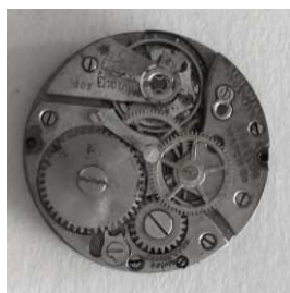
56 SC/120 SC (here the version with three barrel bridge screws)
