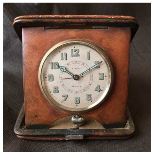
9 - Early foldable travel clock in leather case with eight day movement and alarm, with rare calibre SF-N 100.
