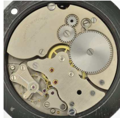
23 - Movement of the airplane clock in picture 23, eight day-calibre SF 190.
