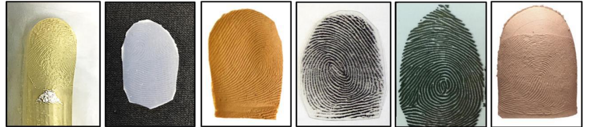
Gelatin Dragon Skin Latex Body Paint 2D Printed on Transparency Conductive Ink on Paper Universal Targets
