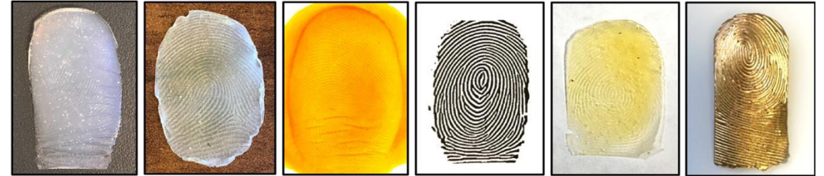
Silicone Monster Liquid Latex Play Doh 2D Printed Paper Wood Glue Gold Finger
