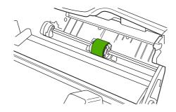
6 Position the new pickup roller in the slot of the previous pickup roller.
