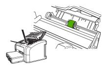
4 Gently release the small, white tabs on each side of the pickup roller by pushing them away from the roller, and then rotate the pickup roller toward the front.
