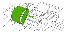
7 Rotate the top of the new pickup roller into position until the white tabs on each side of the roller snap the roller into place.
