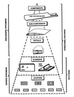
Figure 2 - Schematic diagram of building block tests for a tail rotor blade.
