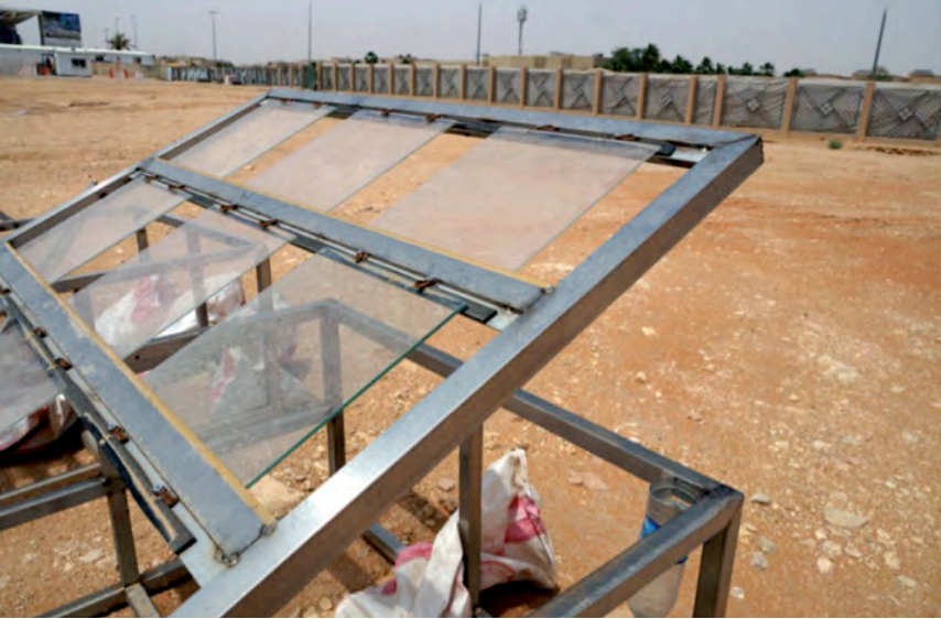
Test-stands for panels with anti-dust coating
