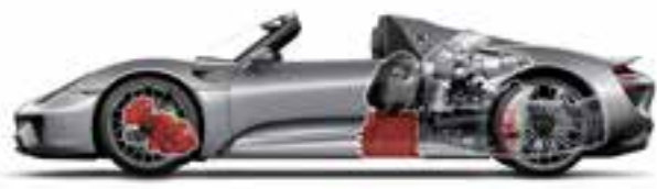
Split drive, low centre of gravity: the 918 Spyder's weight is ideally distributed.
