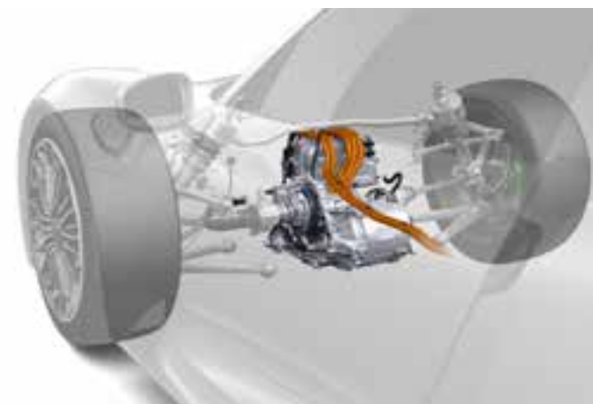
Sophisticated, compact: The additional electric motor on the 919 Spyder’s front axle is a key part of the electric Porsche Traction Management (ePTM) system that gives the car even more traction and driving feel.
