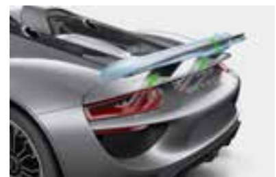
Porsche Active Aerodynamics (PAA) on the 918 Spyder: cooling air hatches, front diffuser and a rear wing can all be adjusted to the specific driving mode.
