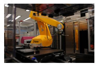
A robot arm at NCATS' Tox21 laboratory retrieves compound plates from storage incubators (right) and brings them to a transfer station (foreground), where compounds are transferred to assay plates using a pin tool.
