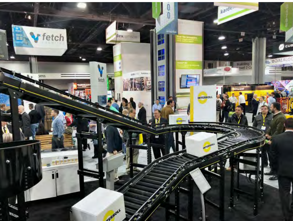
Interroll impressed visitors to the ProMat in Chicago (USA) with inclined belt conveyor modules that save space, particularly in retrofit projects.
