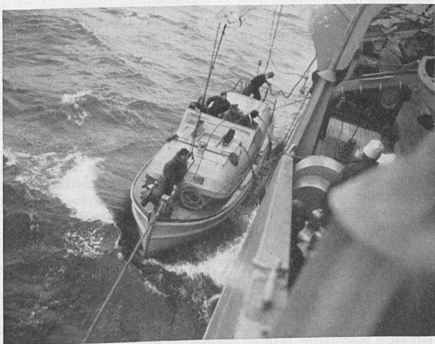
Hydrographic launch being hoisted aboard U. S. C. and G. S. ship Pathfinder .
