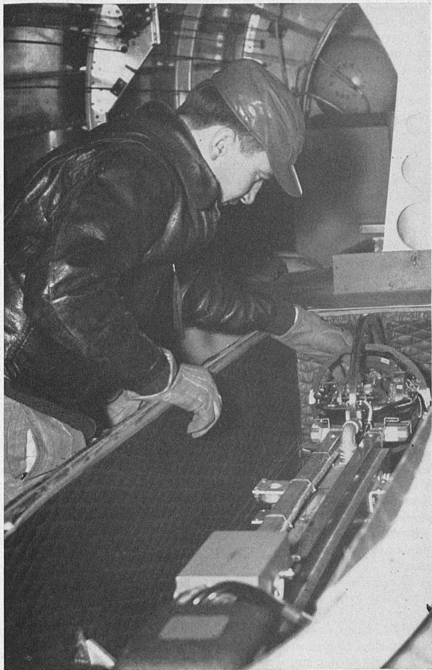
The airborne magnetometer, developed in cooperation with the Naval Ordnance Laboratory, a device of great importance in future magnetic surveying. Installation aboard plane. (Official photo, U. S. Air Force.)
