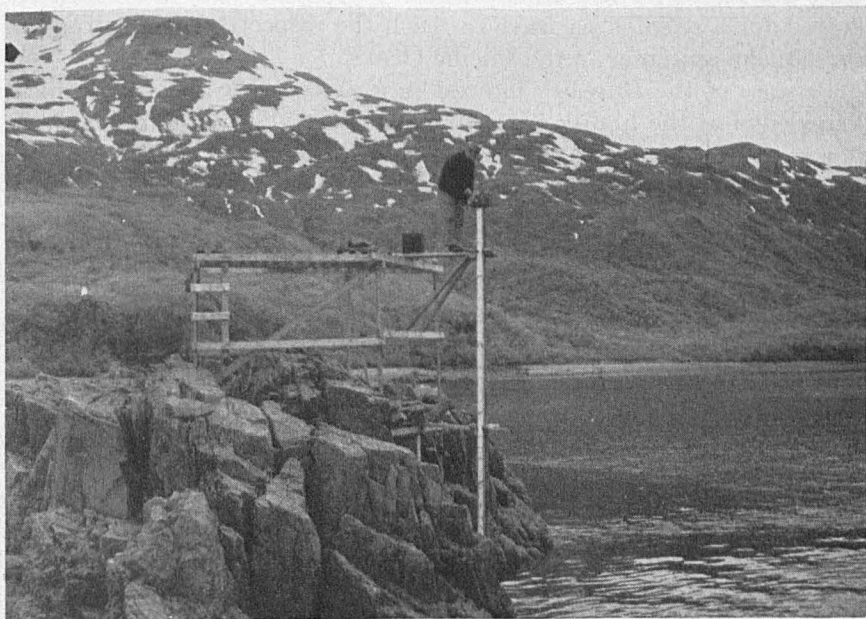
Aguligik tide gage on Alaska Peninsula, used for measuring rise and fall of the tide during hydrographic survey operations in the vicinity.
