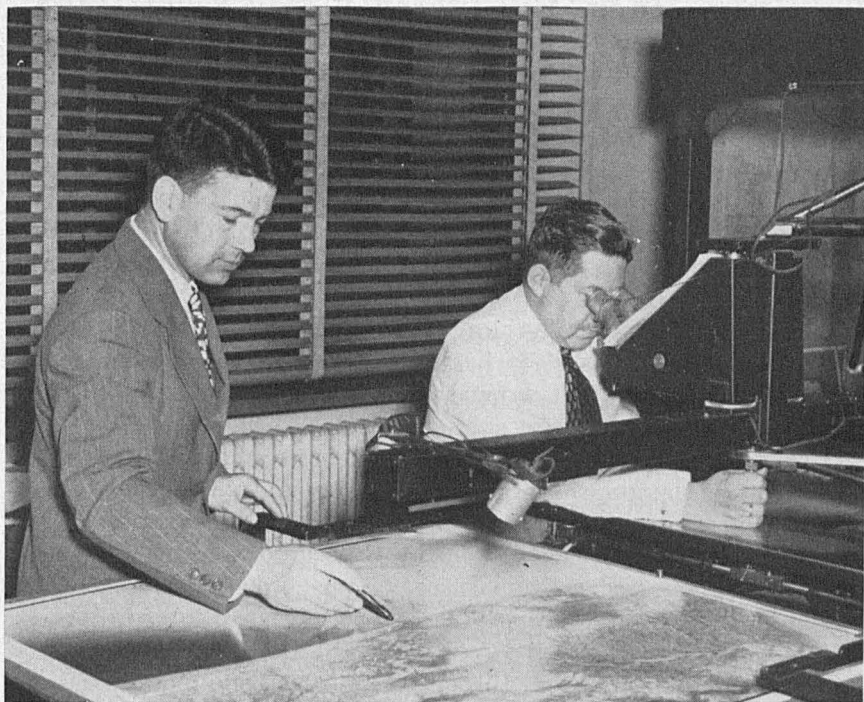
Survey expert in photogrammetry (left) instructing Latin American trainee in the use of the Reading Plotter in compiling maps from aerial photographs.
