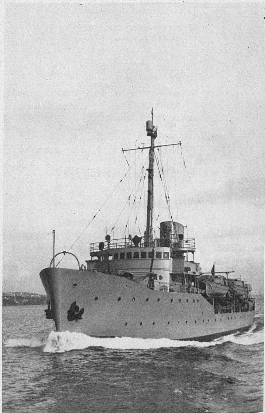
U. S. C. and G. S. ship Pathfinder leaving Seattle. This vessel has a displacement of 2,000 tons. Its over-all length is 229.3 feet, beam 39.0 feet, and draft 15.5 feet.
