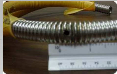
This photo depicts a hole created from excessive electrical current after a lightning strike.
