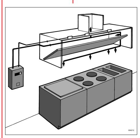
The detection portion of the fire suppression system allows for automatic detection by means of specific alloy rated fusible links, which, when the temperature exceeds the rating of the link, the link separates, allowing the regulated release to actuate.
