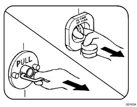
Once the fire suppression system is actuated, equipment to shut off the fuel supply to the cooking appliances will operate.
