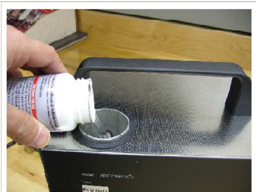
Figure 2. Pouring the treatment into the filling chamber.
