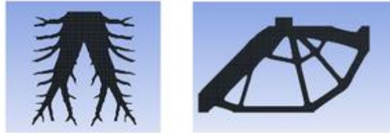
Topology optimization in thermal analyzes (left) and shell structures (right)
