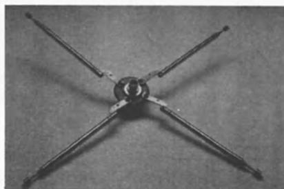
Fig 1—The ground-plane portion of the portable 2-meter antenna. Construction centers on an ordinary steel washer, about 2½ mm thick and 4 cm in diameter.
