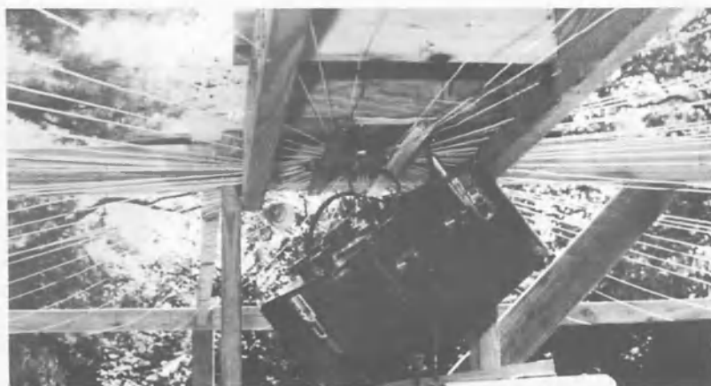
Fig 5—Test equipment was located at the base of the antenna, beneath the counterpoise system. Equipment so located is virtually "invisible" to the antenna itself.
