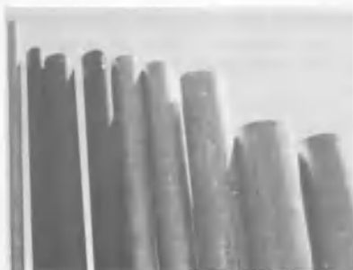
Fig 3—This photo shows the variation of heights found necessary to resonate elements of various diameters at 29.0 MHz. The length difference between the thinnest element (1/8 inch) and the thickest element (2 inches) is 5 inches.
