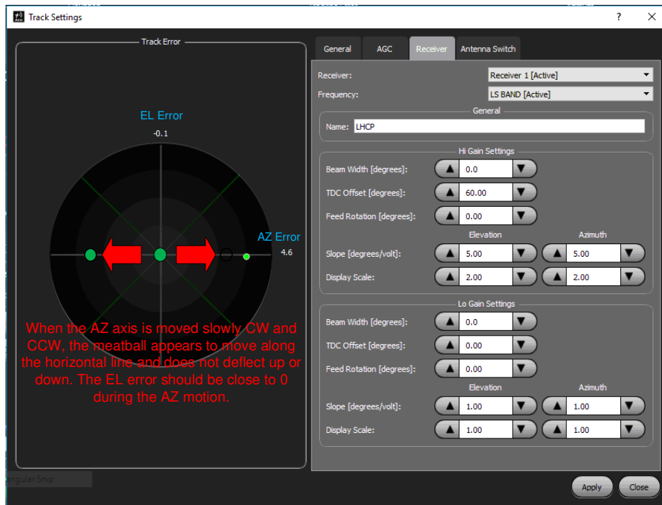
Figure 112: Track Settings Condition 1-Adjusting TDC Offsets
