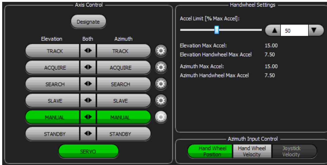
Figure 12: Manual Axis Control with Two Axis Manual Selected and Handwheel Settings Window Open
