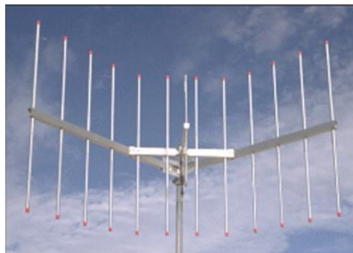
Figure 3-18. Corner Reflector Antenna
