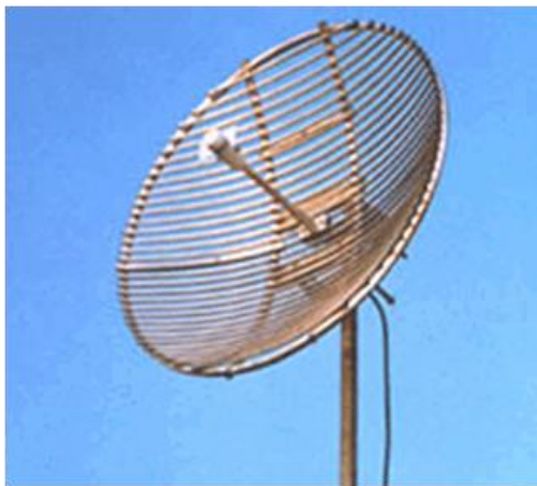
(a) Paraboloidal Antenna
