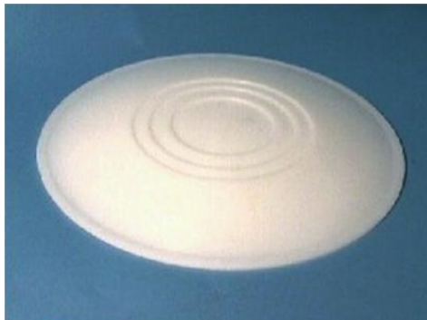
(a) Fresnel Lens (Showing Four Superimposed Lenses)
