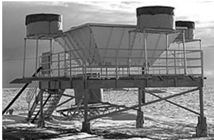
Figure 5-15. 915 MHz Wind Profile Radar for U.S. Atmospheric Radiation Measurement
