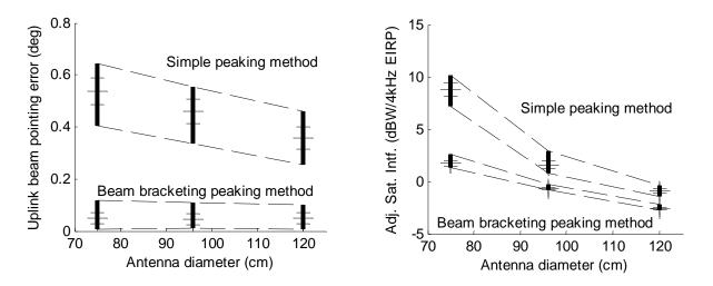
Figure 16. Ku VSAT pointing error and adjacent satellite interference levels.
