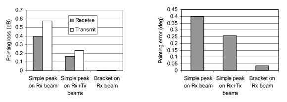
Figure 9. Comparison of pointing methods for a 0.75m Ku-band antenna.
