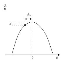
Figure 7. Simple peak pointing method.
