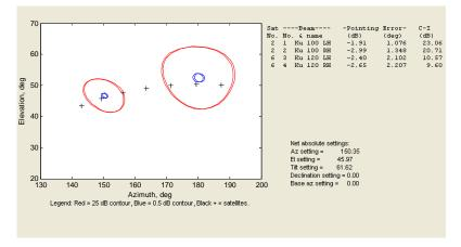
Figure 11. Sky view of an example dual-beam, dual-satellite scenario.
