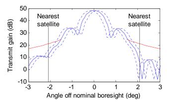
Figure 19. Andrew 4.9m antenna, transmit beam.
