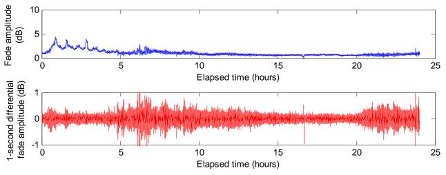
Figure 6. Sample data from the NASA ACTS experiment (20 GHz).
