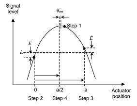
Figure 8. Beam bracketing pointing method.
