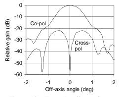
Figure 10. Example offset reflector antenna patterns.
