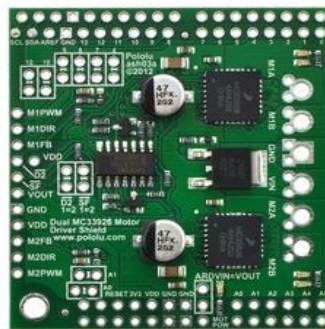
Figure 3.11: Pololu dual MC33926 motor driver shield for Arduino [6]
