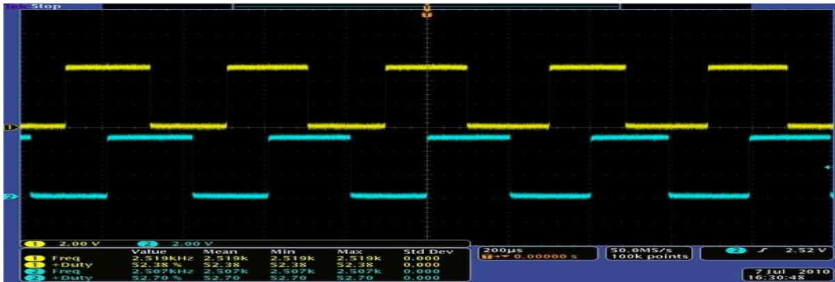
Figure 3.9: Encoder's A and B channels outputs captured through oscilloscope [6]
