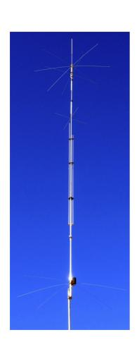
• Elevated Vertical: omnidirectional, narrow Bandwidth, optimum mounting height 18', efficient with 3 to 4 tuned elevated radials.
