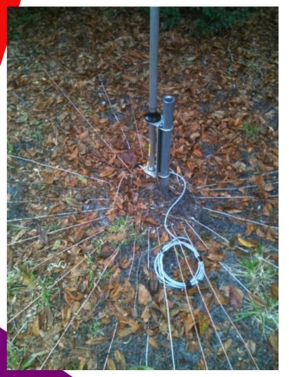
• Ground mounted Vertical: Omnidirectional, efficient with large ground radial field.
